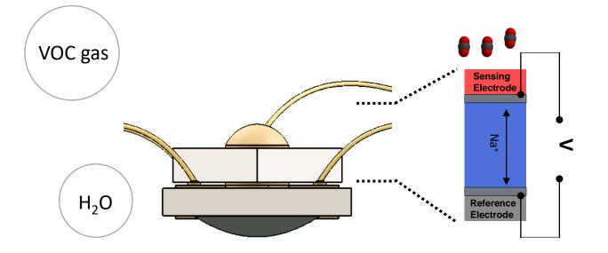
Under non-operating, VOC gas and H<sub>2</sub>O gas could adsorb to sensor. Because the sensor is ceramics it have very many pores can keep the gas. So when operate the sensor again. It may needs the time to heat to remove the gas from sensor. After the burning the gas on the sensor, sensor will be operated properly. It takes time about 1 or 2 days to burn it. so storage the sensor under dry and clean atmosphere.
